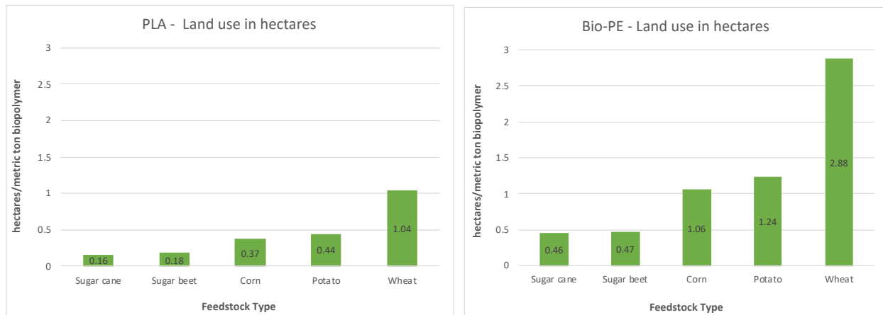
Land use comparison of sugar cane, sugar beet, corn, potato, and wheat for the production of PLA and Bio-PE, data from Institute for Bioplastics and Biocomposites, 2019
